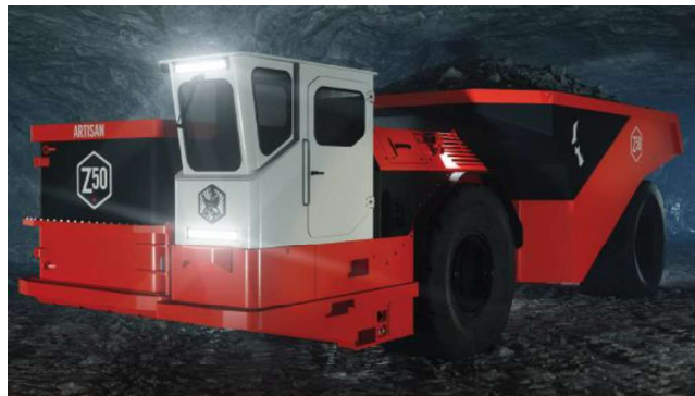
Figure 26 - Artisan Vehicles® Z50 (Artisan Vehicles, Battery electric 50 tonne haul truck, nd a)
