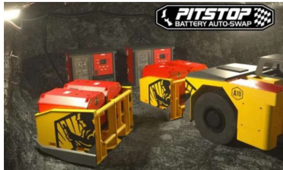
Figure 33 - PitStop Battery Auto Swap (Artisan Vehicles, 2019)
